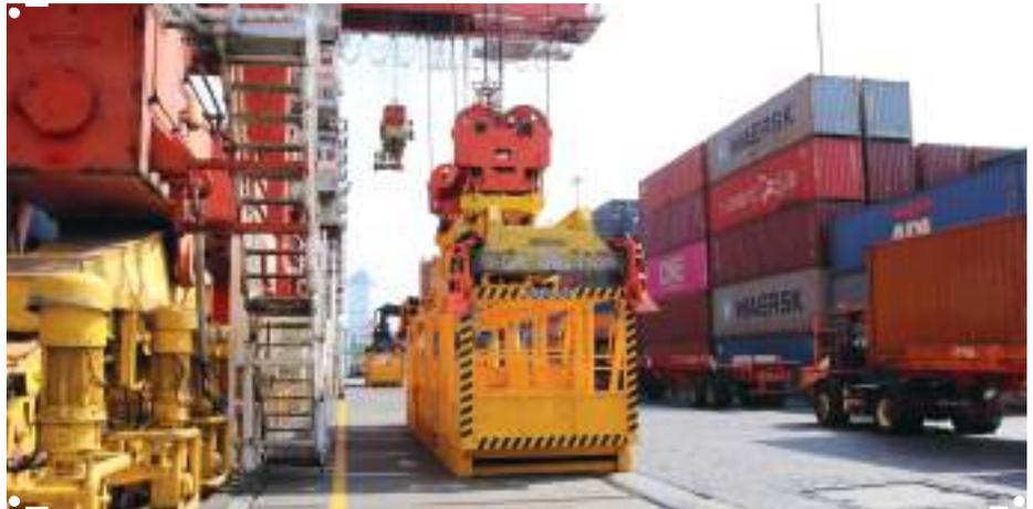
**SAGT commissioned two Container Top Safety Work Cages (CTS-WC) to enhance the safety of its container lashing crew for operations on board.**
